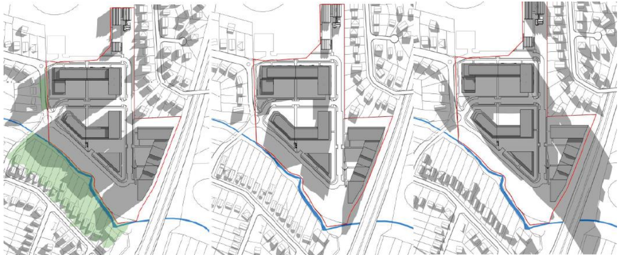
Figure 10. Diagram showing the extent of overshadowing from the proposed scheme at 9am, 12pm and 3pm on 21 June (Source: Applicant's planning proposal)
